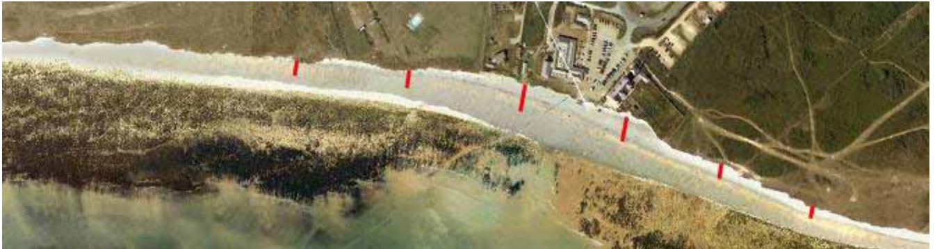
Figure E8.1 Shows the locations of the 2008 transect surveys carried out at Birling Gap beach.
